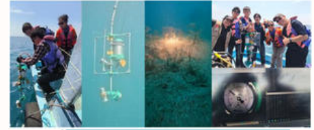
Gambar 31. BASSCAM: Bathyal Area Scouting Subsea Camera
